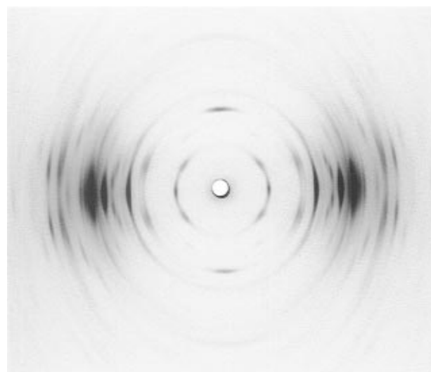
Figure 7. X-ray diffraction pattern at room temperature of a fiber sample of P(2,1) annealed for 3 h at 180 °C (phase I + phase II).
